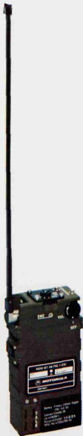
This AN/PRC-112(V) lightweight survival transceiver is designed to locate crews of downed aircraft.
