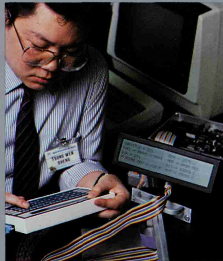
Software engineer uses universal calibration console, which displays engine performance parameters under on-road conditions, to calibrate and test electronic engine control modules.
