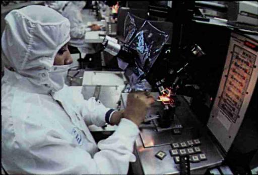
Technician assembles an MC68020, the 32-bit "mainframe computer on a chip."
