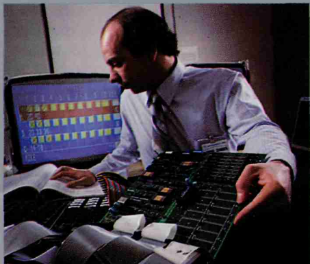
Functional testing of a custom-developed bit-mapped graphics subsystem.
